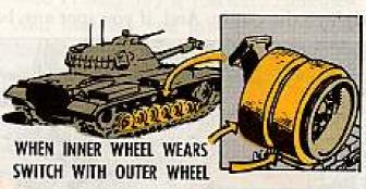
When you notice your inner roadwheels are wearing down, switch the inner and outer wheels to equalize the wear and give 'em a longer life.
