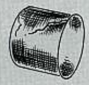
FUEL TANK FILTER STRAINER —Dirty. Damaged screen.
