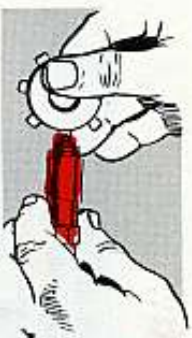
SPARK PLUG —Insulation cracked; points burnt, carboned, pitted. Gap out of adjustment.
