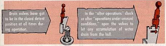
Before you park for the night the valves have got to be left open to drain off any rain or snow or any fuel or oil that might leak during the night.
