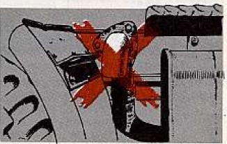
point down, and here's why. Turning 'em up like you suggested might increase the fire hazard. It would mix heavier-than-air exhaust fumes with lighter-than-air gasoline fumes coming from the vent in the gas tank cap.
