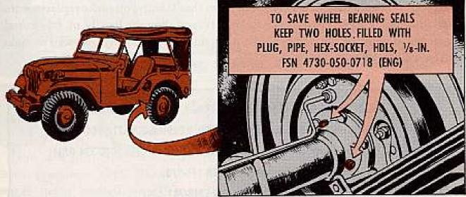
Your LO calls for cleaning and repacking the bearings with GAA every 12,000 miles or annually. You'll need to dis-assemble 'em to do the lube job and to make sure that no grease is on the brake linings.
