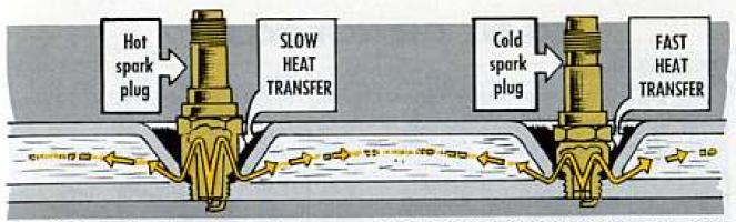
ferred from the plug, through the engine block, and into the cooling-system liquid. The plug has to stay hot enough to hold down carbon deposits, but not get so hot it'll cause pre-ignition, or knocking.
