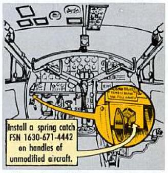
If you're twisting a wrench around one of these, look up item eight under project 59-1888 in TB AVN 23-5-9 (29 Sept 59). It supersedes the entry under project 58-4438 in TB AVN 23-5-1 (1 Jan 59). The later copy of the UR Digest passes the word to install a spring catch, FSN 1630-671-4442 (P/N C3CF603-11), on the handles of the unmodified aircraft.
