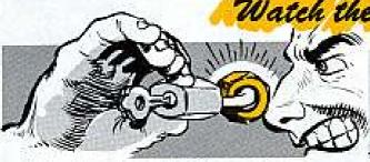
The jam nut which keeps the elevating jack screw bearing tight in the M13 cupola of your M59 personnel carrier or M84 mortar needs to be looked at at every Q service for tightness.
