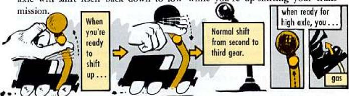
After your shift, pull the button back up, or right, and when you're ready to shift the axle up, release the clutch and throttle again. You do the same thing for your shift from second to third. Push the button down, or left, and then make your shift in the regular way. Then pull the button up, or right, again and slack your throttle when you're ready for high axle.
