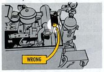
Stand by the generator and face in the same direction as the starter rope end of the generator. Then take a look at the rope. If it comes out of the shroud like above, the rope'll bind against the shroud when you pull on it. The rope wants to come through the other shroud slot . . . and here's how you get it to work that way.
