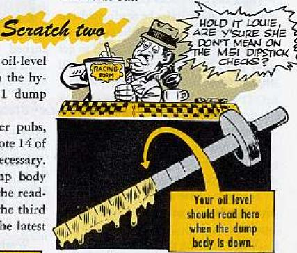
One of the readings used in the past ... with the dump body up on the safety braces...could be dangerous. 'Specially if the control lever got left in POWER-DOWN instead of being shifted into NEUTRAL.
