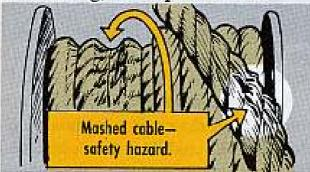
Say you've got a heavy job coming up. The strain is heavier—a lot heavier—than last time, and the outer wind of tight cable will be mashin' itself through those loose layers. After a gnawin' like that the cable's a real safety hazard.
