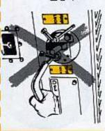
wrench or pliers—too much pressure will damage the needle and trol—are closed to linger lightness. Lay off tightening them with a valve seat. 1. Make sure the metering valve levers—there are two on each con-
