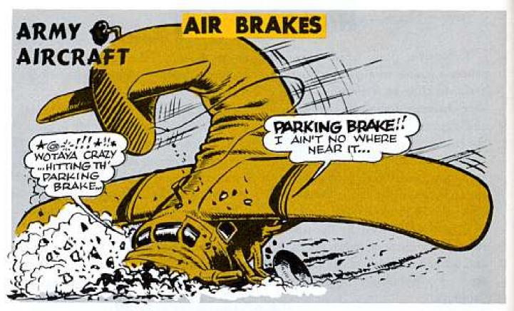
Some of those Otter (U-1A) parking brake handles have a nasty habit of vibrating into the locked (ON) position when you're not looking. Then, while your favorite flyboy is roaming around the wild blue yonder, thermo expansion of the red juice in the brake system locks the brakes—same as if the toe brakes had been hit while setting the hand brake on the ground.
