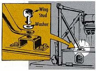
slack in the stud by slipping a flat washer over the stud (stud remover) and over the hold-down pin, then put the stud back into the bracket and get the whole works tied down good'n snug so that it takes a pair of pliers (almost) to turn 'em.
