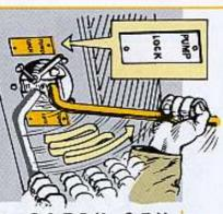
2. To lower a corner of the trailer, turn the selector valve handle for that corner to PUMP—turn the other selector valve handle on the control to LOCK.
