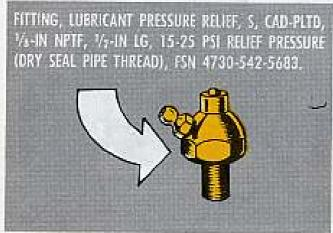
If your vehicle had either MWO Ord G1-W106 (15 Aug 57) or MWO Ord G1-W106 (27 Jan 58) installed, all you'll need to do the job is the new fittings and bushings (FSN 4730-141-9098) on opposite side of the roadwheel hubs and compensating idler wheels and arms.
