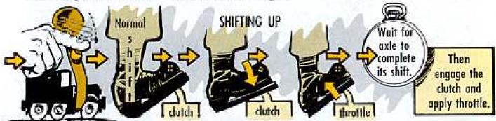
Before shifting to first to start out with a load, you push the button down, or left, then start off in the usual manner. Then, when you are ready to shift the axle from low to high, push in on the clutch and release the throttle and wait until the axle completes its shift, and then engage the clutch and apply the throttle.
