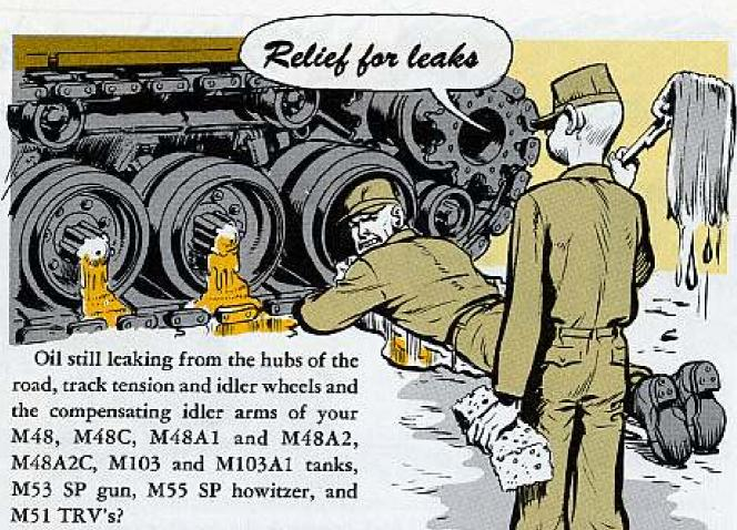
This leakage was supposed to be dried up by application of MWO Ord G1-W106. It called for replacing the pipe plugs with lube fittings and use of GAA amendment 3 instead of oil.
