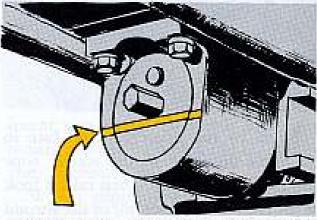
If the parts inside the block are installed right, the cap'll stay put and the yellow line'll be straight.
