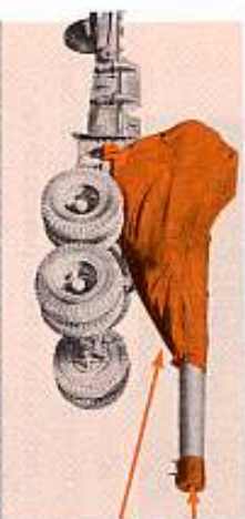
AIR BRAKE HOSES —leaks, cracked, connectors broken, connector gasket damaged, painted or missing.
