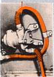
AIR BRAKE HOSES —leaks, cracked, connectors broken, connector gasket damaged, painted or missing.
