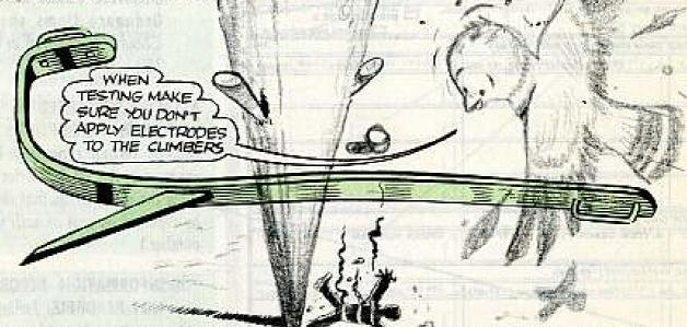
If a support outfit near you has 'em, Magneflux machines should be used to check out those climbers. If flaws are detected . . . or your climbers have a zinc or phosphate-coating . . . turn 'em in pronto.
