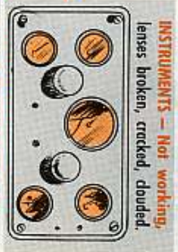
WATER TEMPERATURE GAGE —Lens cracked, dirty, clouded. Doesn't work right (temperature should read between 160°F and 180°F when engine's warmed up).
