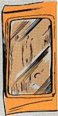
REAR WINDOW —Fogged enough to hamper vision, ripped.
