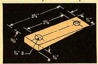
If no scrap bar stock is available, then try supply for Steel, Mild Carbon, (SAE WD 1020) Bar, Flat, 1/2 inches, FSN 9510-596-2285.
