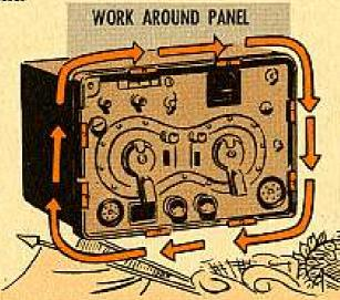
The danger lies in tightening up only one or two fasteners before the others are lined up and ready for final adjustment. That actually takes extra effort on your part and, worse still, puts a mighty heavy strain on the one or two Dzus's that were turned tight before the others.
