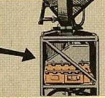
Hard to believe, but the lubricating oil (GO 90) in the base (AB-221/TPS-1D) gets gummy and dirty and soon clogs the gears—leaving you with a sick Tipsy Dog.
