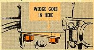
When it comes to hooking them up again, the two front mounting bolts will hafta be swapped for new ones. Get supply to give you Bolt, Machine, Hex-Hd, Low Carbon-S, Cd or Zn pltd, 3/8-24NF-2x1. These bolts are long enough to make up for the difference taken up by the spacer. Of course, you've gotta keep the nuts and washers, so you can reuse 'em.
