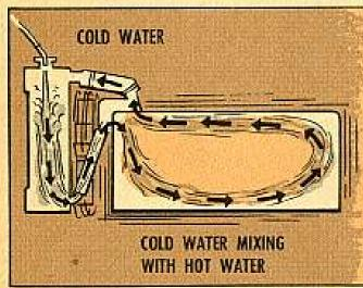
Now, when you do go to pour water in, make sure the engine's running. This lets the water pump force warm water from the block up the radiator inlet hose. The cold water you add cannot run into the hot engine, but must first pass down through the radiator, mixing with the warm water being forced up by the water pump. This means that warmer water passes into the block instead of cold. Makes things safer.
