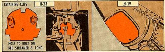
So we've made up a set of covers for the openings in the tails. We put 'em on when we tie down, and remove 'em before flight. The inclosed sketch will show you what I mean.
