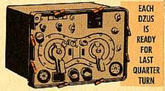
And then work right around the panel making the final, quarter-turn adjustment.
