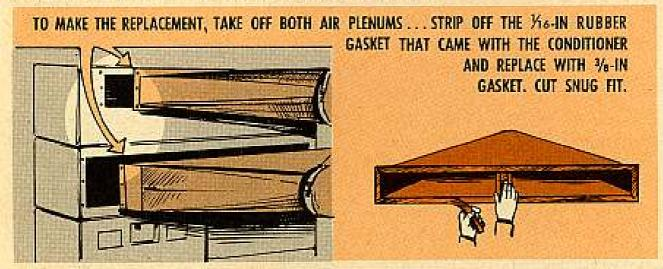
Cut the gaskets at the corners for a snug fit. Then you give it a coat of rubber cement to make sure you have a good seal before you put the plenums back in place.
