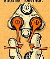
**WORK PRIMER AS ENGINE IS** TURNING OVER, AMOUNT OF PRIMING DEPENDS ON HOW COLD YOUR ENGINE IS.
