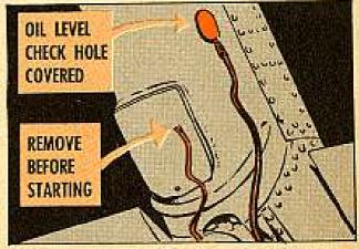
before starting" red streamers attached to the covers and fastened to the aircraft whenever the plates are in, to remind the crews to take 'em off.)
