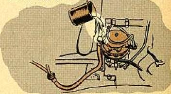
in the fuel system and caused the lock. Of course, if there's no water around, you'll have to wait for things to cool off inside that engine before you can start it.
