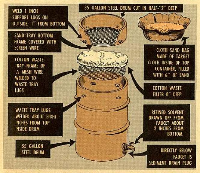
To test the filtration unit we used dirty cleaning solvent that'd been used in the shop on bearings coated with grease, dirt and rust—the gookiest we could find. Yet it came out clean and clear. In fact, based on the results of this test, we figure to reduce waste of cleaning solvent around here by 75 per cent.
