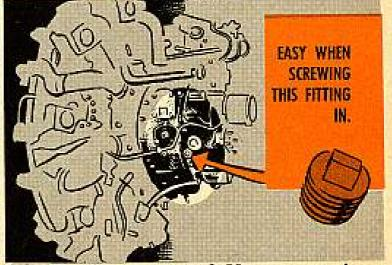
But, that's not only all you need—it's all you can stand. You are screwing a tapered plug into an aluminum alloy housing, and it doesn't take much to bust the housing. It's like driving in a wedge to split a log.
