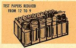
of the paper packets with chemicals in 'em have gone modern—the chemicals are now packaged in glass and pelyethylene tubes. Keeps 'em pure and dry.
