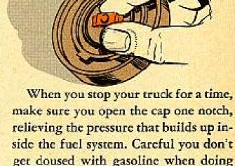
this. Tighten the cap again before taking off on another run. To get the lowdown on this gas-tank cap and how to use it, read over your copy of TB Ord
