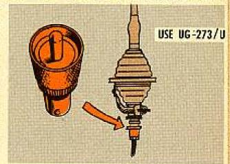
This adapter can handle the ground strap from the mast base without interrupting the circuitry. Just clamp the strap to that adapter and you're grounded just right.
