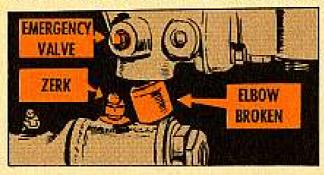
There should be about ½ inch leeway twixt the lower edge of the elbow and the top of the lube fitting, but this could vary somewhat. If there's clearance, you've got no problem. But if you have no clearance then the air tank gets a shimming job—done with two homemade spacers.
