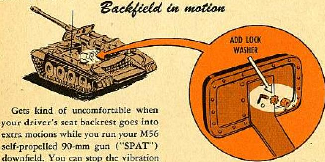
from loosening the backrest by putting on a lockwasher...like the new models are getting. It'll hold better than a grade-A girdle.
