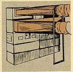
To keep your dual installation of the BAF-55118 equipment air tight, you'll need 31 feet of 3/8-in x 11/4-in rubber gasket. Fourteen feet, 1 inch will go for the discharge plenum and 16 feet, 81/2 inches for the return plenum. Order the rubber from your direct support unit (Jarron Products Co., part number C510-310, or equal will do the trick). It's a local purchase item.
