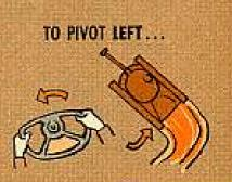
LET THE ENGINE DROP TO IDLE (650 RPM) WHEN PIVOTING, THEN CONTROL YOUR TURN WITH A COMBO OF YOUR GAS PEDAL AND PRESSURE ON THE WHEEL.
