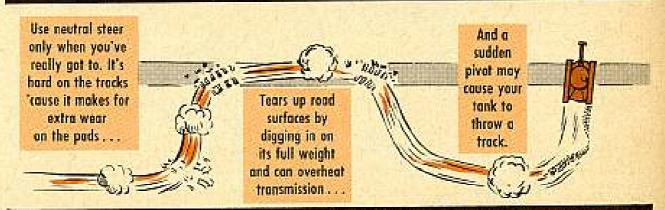
IN NEUTRAL STEER, THE CROSS-DRIVE TRANSMISSION WILL CAUSE THE TRACK TO TURN BACKWARD WHILE THE OTHER TRACK TURNS IN THE OPPOSITE DIRECTION.
