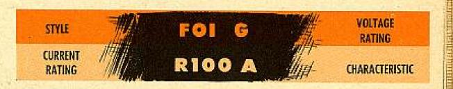
Either way it means the same thing. This particular one translates to a Style F01 fuse, with a G voltage rating (250), an R100 current rating (0.100 amps) and the A characteristic, which means it has normal interrupting capacity (not a slow-blow, and not a special high interrupter).
