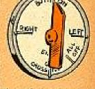
Turn knob to either RIGHT ON or LEFT ON. After engine's warmed up, you can put it on BOTH ON. Electric fuel pumps cut out and the main engine pumps take over in the BOTH ON position.
