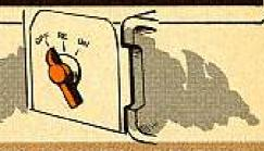
SHUT OFF ALL LOAD SWITCHES ... TURRET POWER, VENTILATOR, FIRE CONTROL. HEATER EMERGENCY SWITCH MUST NOT BE USED TO TURN OFF PERSONNEL HEATER. THE HEATER WILL BURN OFF (PURGE) WHATEVER FUEL IT'S GOT AFTER IT'S BEEN SHUT OFF, SO DON'T THINK YOUR HEATER'S FLIPPED ITS LID. IT'S NOT A GOOD IDEA TO RUN HEATER WITHOUT ENGINE OR LI'L JOE WORKING 'CAUSE IT PULLS PLENTY POWER OFF THE BATTERY.
