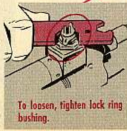
For removing sear release.
