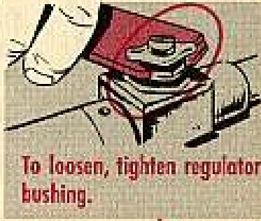
To loosen, tighten gas screw regulator locking nut.
