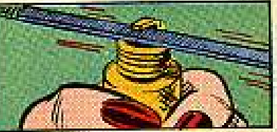
Open the gap enough to get an ignition point file or stone in.
