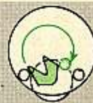
turn the latch knob clockwise by hand to put the latch in position to receive the latch pin.
