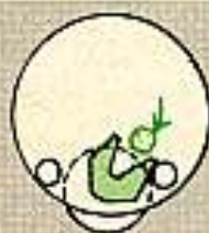
The second time around, the pulley will hit the latch against the stop pin . . .
