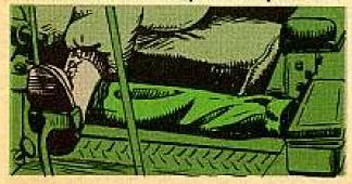
This cover can be put on and removed in a few seconds. When it's stowed, it's out of the operator's way and doesn't interfere with any of the controls. All it takes to make it is canvas and some scrap metal.
