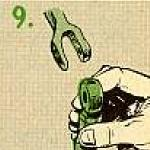
Disconnect the next rod, which is the long vertical job leading from the first bellcrank to the turret floor. Loosen it at the end of the bellcrank you just pinned.
