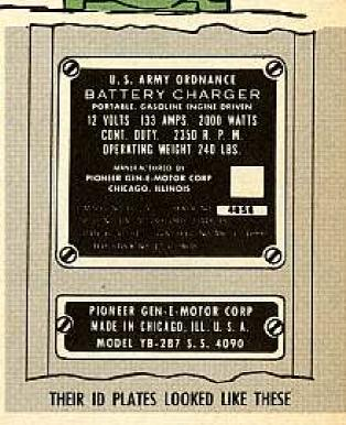
Then along came SM 5-1-6100 (May 1956) and things were changed. Both models became Model BC-20L-SS-4090, and both Engineer stock numbers were converted to FSN 6115-635-6625. New ID plates were called for.
