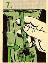
Disconnect the rear of the short horizontal rod at the bellcrank located behind the shift quadrant.
