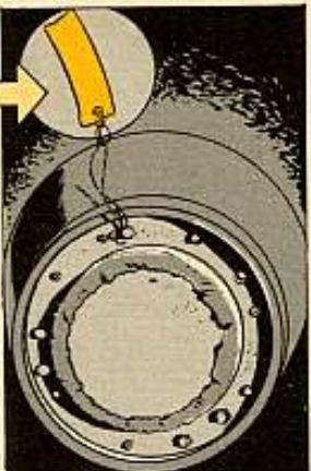
MISSILE IDENTIFICATION TAG PROPERLY ATTACHED TO AFT END OF MISSILE
