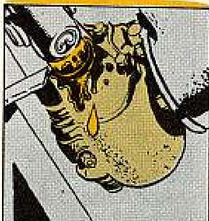
POWER TAKE-OFF UNIT —lube leaking (not a seep)
