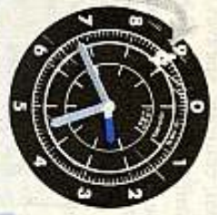
The little hand gives you a 1000-hour reading on the little, inside track.
