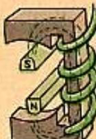
This flux passes through turns of primary and induces current in coil.
