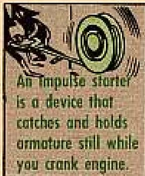
An impulse starter is a device that catches and holds armature still while you crank engine.
