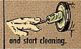
When you're done, wipe away the compound with lens paper that has been folded twice. You fold the paper that way so's oil from your skin doesn't get through to the lens. Rub from the inside outward, and change the paper once in a while to get rid of any grime that collects on it.
