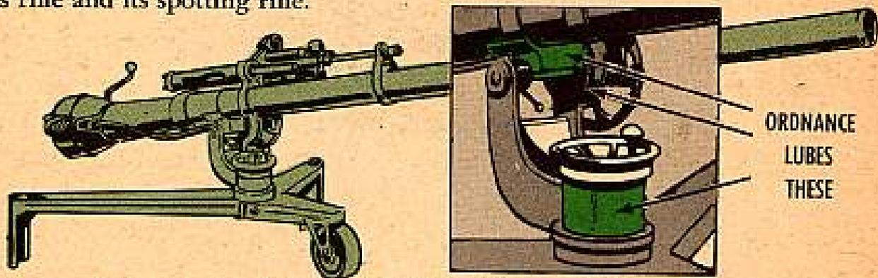
Pay real attention to "Note 5" which tells you Ordnance shoots GL in the elevating and traversing mechanisms and the firing transfer box on the 106. This is done when the weapon is disassembled—or about every six months.
