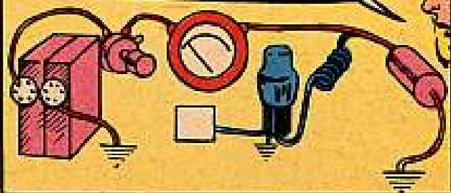
Here's a thumbnail of how it works: the dry cell batteries send current through meter to charge condenser.
