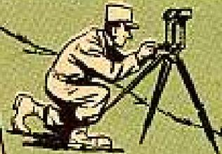
Do spread the legs and embed the feet in the ground. If the legs can be extended, adjust them so the head is level. On a slope, put two legs on the downhill side. Keep the extension leg clamps tight.
