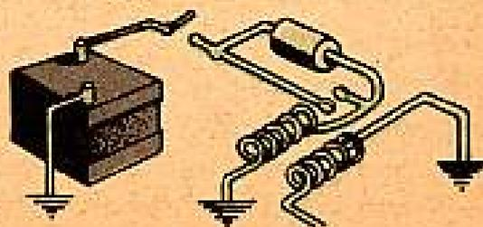
Booster current of about 400 volts is applied to magneto primary winding via ground lead.
