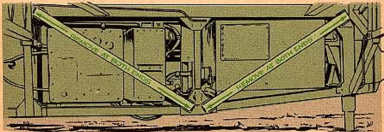
What we did was mark the braces with the words "Remove at Both Ends." Haven't had a bent brace since.
