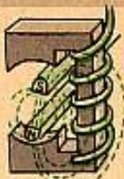
Magnet revolves and sets up moving flux in core.
