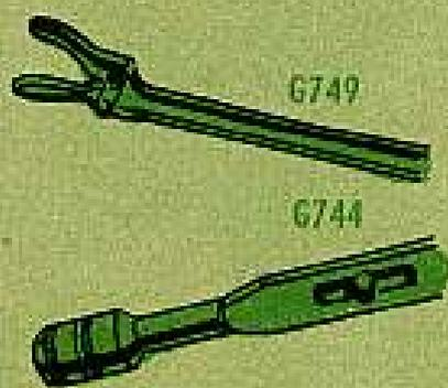
On your G749 2½-ton (TM 9-8024) and your G744 5-ton (TM 9-8028) trucks if less than 1/3 of your handbrake lever is in reserve when you pull it up, the brake needs adjusting. It's best to test the brakes for these trucks when they're on an incline of some kind.
