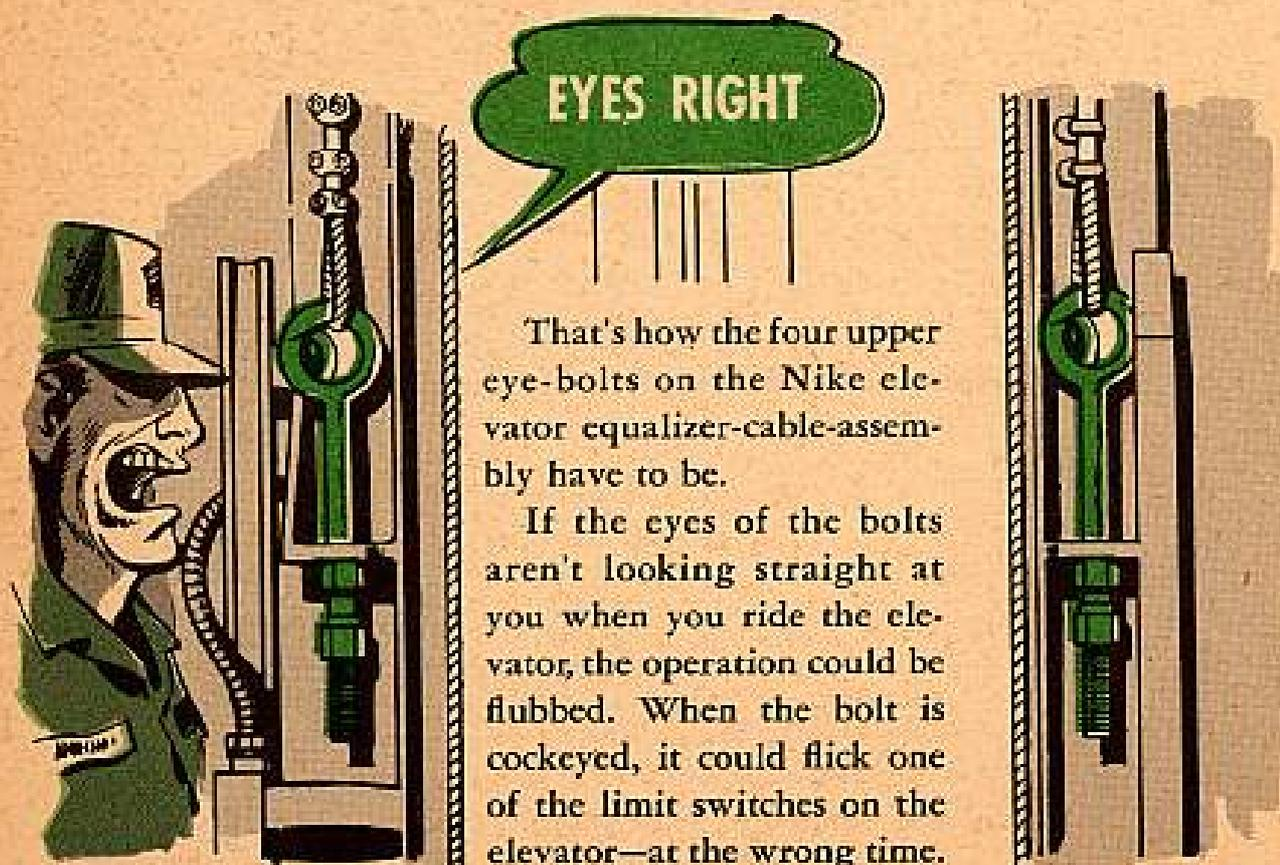
That's how the four upper eye-bolts on the Nike elevator equalizer-cable-assembly have to be.
