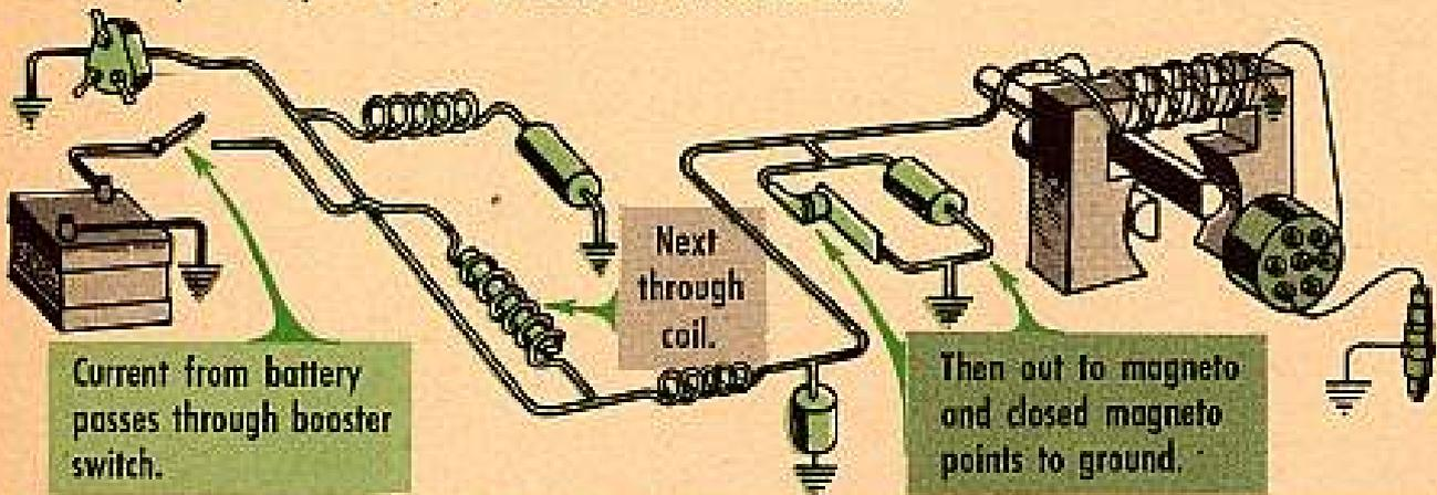
Current from battery passes through booster switch.
