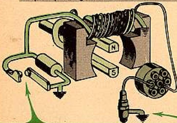
One end of the secondary runs to the center contact of the distributor section of the mag.
