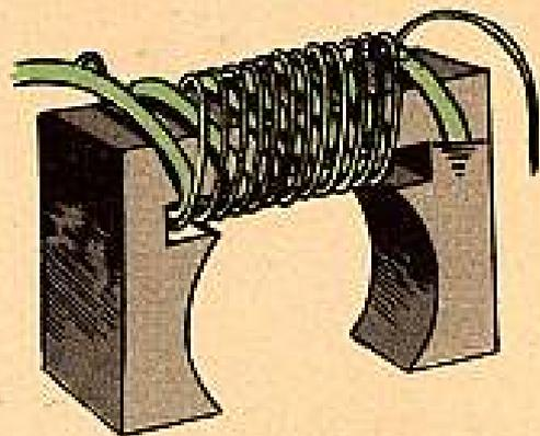
The other end of the secondary winding is grounded. It is grounded through the primary windings, here.
