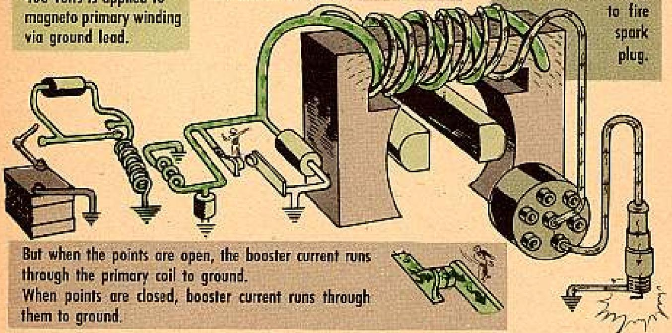
But when the points are open, the booster current runs through the primary coil to ground. When points are closed, booster current runs through them to ground.
