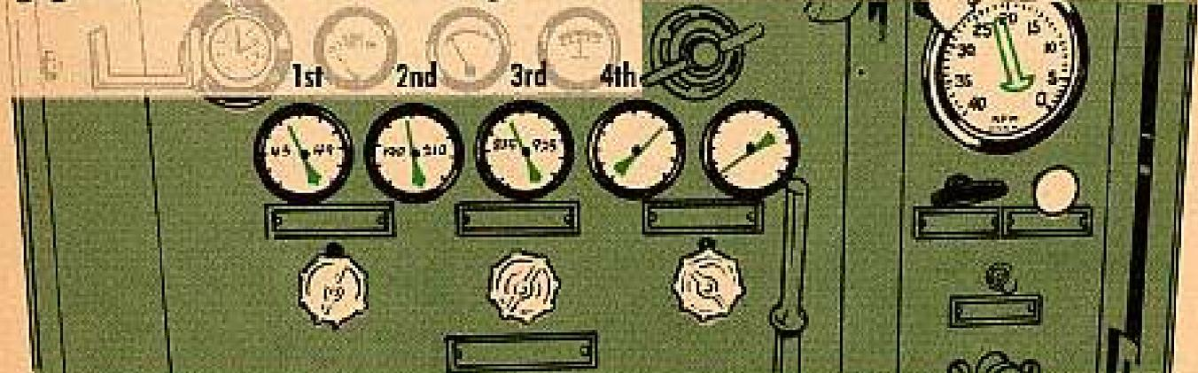
Naturally, the readings won't range that all the time. For the first ten hours of operation on a new Joy (or the next ten hours if you've already got one), jot down the readings in the first three stages when the compressor's fully loaded. Once you've established an average reading, it shouldn't vary more than 3 PSI in the first stage; 10 PSI in the second stage, or 50 PSI in the third stage.
