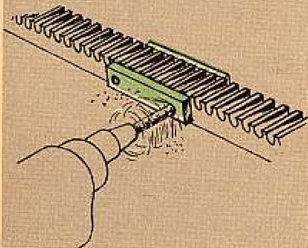
2. Cut two strips of rubber  $\frac{3}{8} \times \frac{3}{8} \times 1\frac{3}{8}$  inches and drill holes in each strip to match the holes in the metal stops and in the rack.
