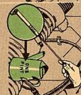
When the reading is just barely on the tip of the dipstick, she takes a pint. You get an idea of how much oil to put in after adding a couple times.
