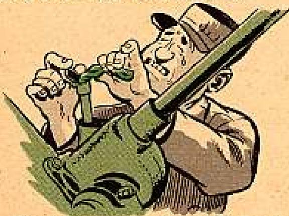
What they'll do if they find grease is to get it out of there and fill the box with either commercial multi-purpose gear oil or military universal gear lubricant (GO).
