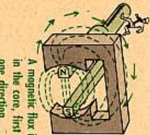
A magnetic flux is set up in the core, first in one direction...
