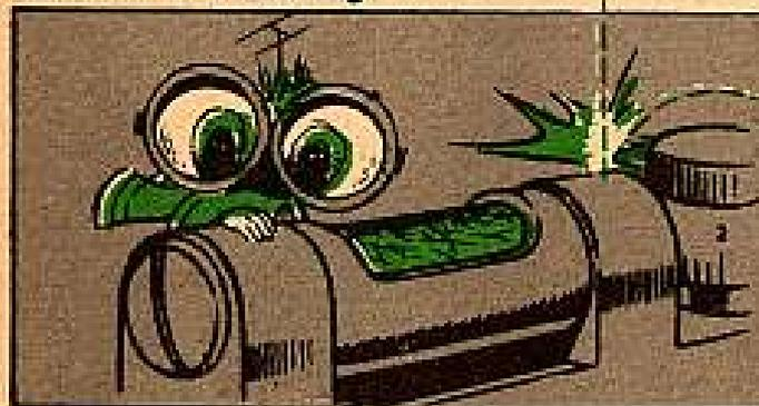
Let's not forget that you also want to use care in cleaning leveling vials. After all... scratches on the vial glass'll make it harder to see the leveling bubble.
