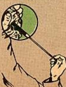
After you add oil—no matter how much—take a dipstick reading to make sure the compressor crankcase is not over-filled. If she is, drain her down to the dipstick full mark.
