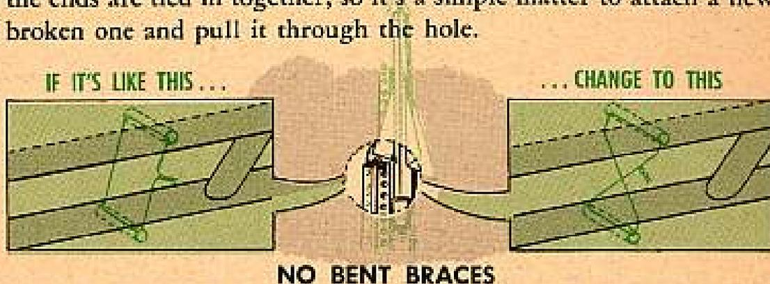
Another idea—one that is saving wear and tear on the elevator platform launcher. It keeps the diagonal braces at the forward end of the launcher from getting torn up.
