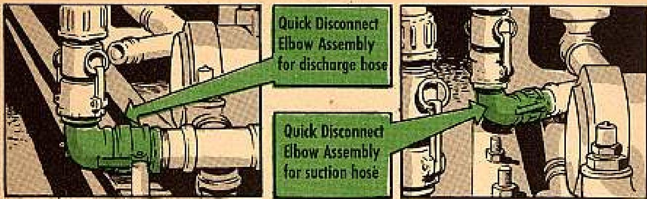
Assemble the two quick-disconnect couplings to the elbow. This makes up the elbow assembly which connects between the inlet connection and the suction hose, or between the outlet connection and the discharge hose.
