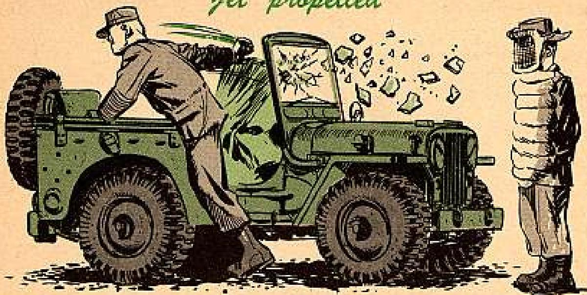
Cases of busted windshields in the M38 and M38A1 Jeeps have been popping up. Reason? Guys crawling into that back seat are swinging the assistant driver's seat forward with all their might—right into the windshield.
