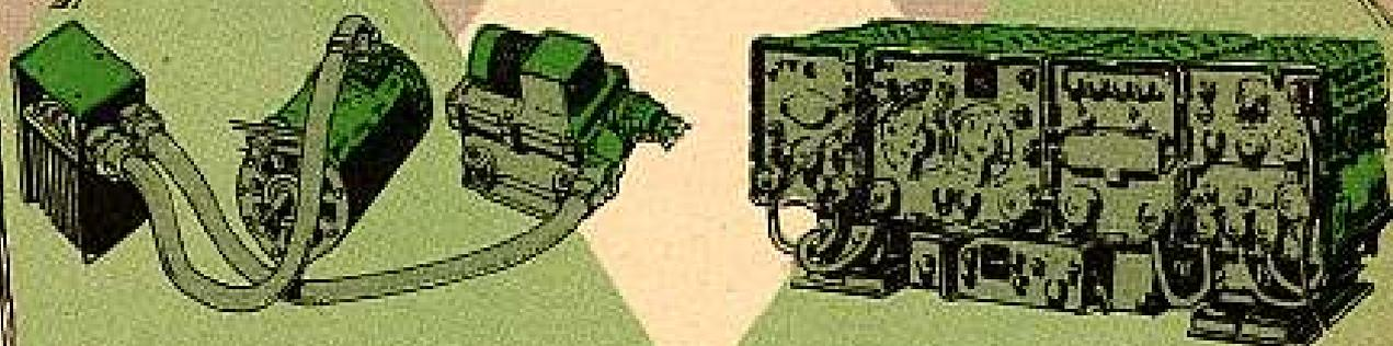
You just can't get the best from a radio set inside that truck of yours unless you have one of these new-fangled AC-DC 100-ampere generating system—the official nomenclature is: **Kit, 100-ampere, 28-volt, rectified AC-DC, generating system.**
