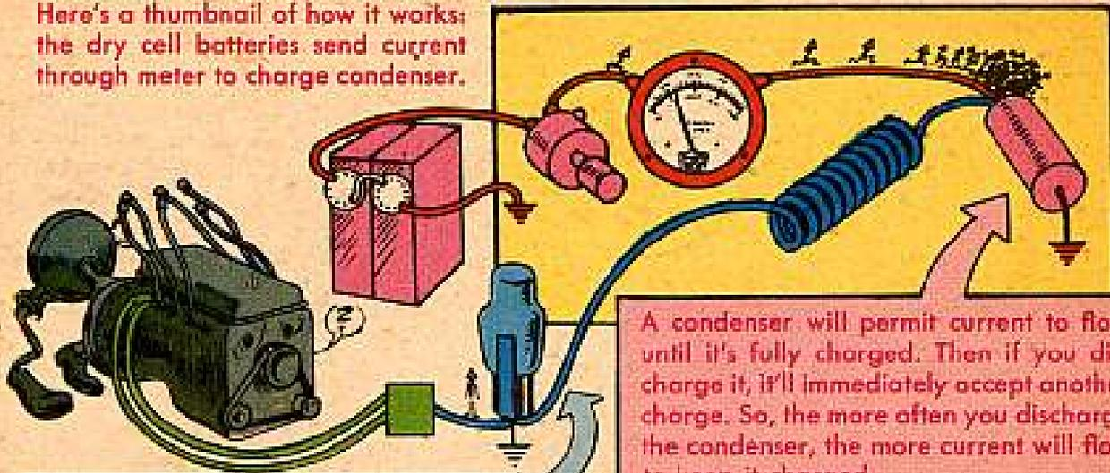
A condenser will permit current to flow until it's fully charged. Then if you discharge it, it'll immediately accept another charge. So, the more often you discharge the condenser, the more current will flow to keep it charged.
