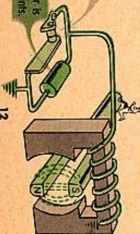
One end of this coil is grounded to the core.
