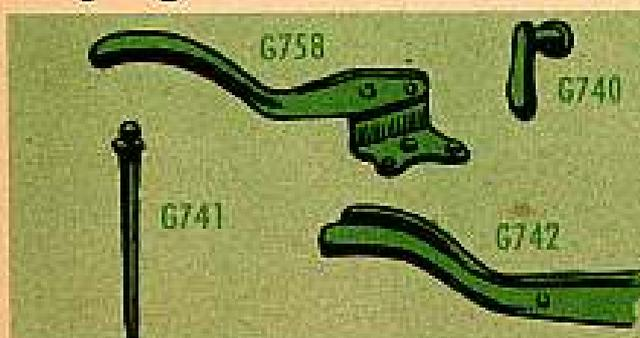
A handbrake adjustment is required on your G740 Jeep (TM 9-8012), on your G758 Jeep (TM 9-8014), on your G741  $\frac{3}{4}$ -ton truck (TM 9-8030) and on your G742  $2\frac{1}{2}$ -tonner (TM 9-8022) when the handbrake lever requires more than  $\frac{3}{4}$  travel for full application
