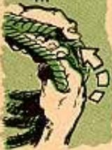
COIL CABLE-LAID COUNTERCLOCKWISE
