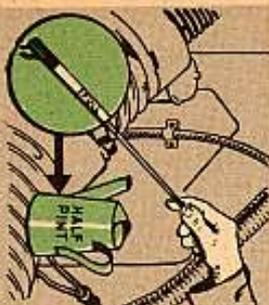
If the reading is halfway between the full mark and the bottom of the dipstick, add half a pint of oil.
