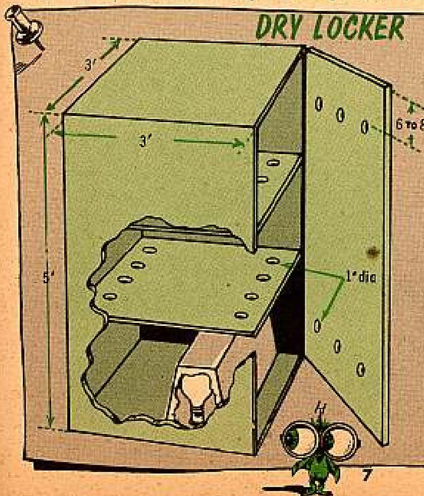
Drill three 1-in holes 6 to 8 inches from both the top and bottom of the cabinet. Drill 'em on either the front or back side — the front being where the door is.
