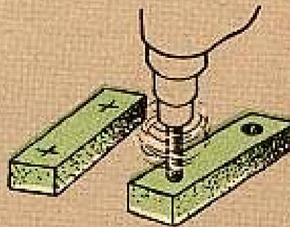
3. Sandwich the rubber strips between the rack and the metal stops. Run a rivet ( $\frac{1}{8} \times 1\frac{1}{2}$ -in round-head rivet) through each hole. Head the rivets for a sure hold, and that's it.
