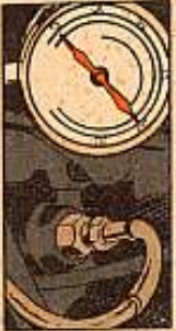
Connect hose of gage into opening
