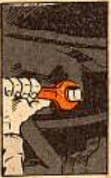
Take out pipe plug at top of intake manifold
