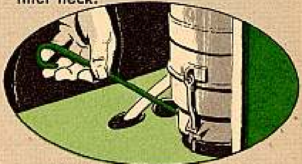
BOTH TRANSMISSION OIL LEVELS
