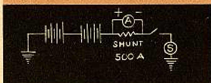
FIG 7—Hookup for starter-motor amperage-draw test.
