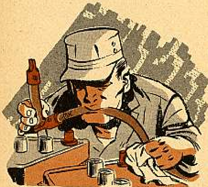
FIG 5—Hookup for ground-circuit cable test. If you get no reading in the 50-volt hole, take the lead out and put it in the 1-volt hole.
