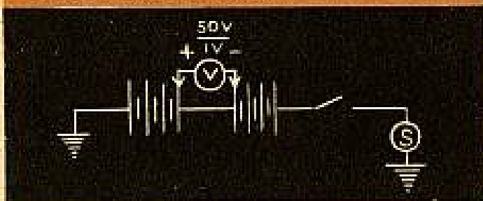
FIG 4—Hookup for battery-jumper cable test. If you get no reading in the 50-volt hole, take the lead out and put it in the 1-volt hole.
