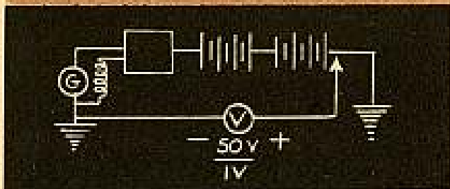
FIG 10—Hookup for charging-circuit ground-resistance test. If you get no reading in the 50-volt hole, take the lead out and put it in the 1-volt hole.
