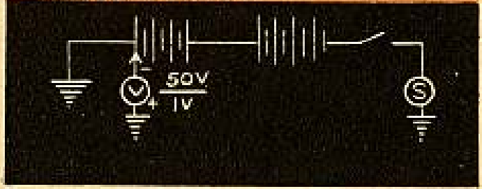
FIG 5—Hookup for ground-circuit cable test. If you get no reading in the 50-volt hole, take the lead out and put it in the 1-volt hole.
