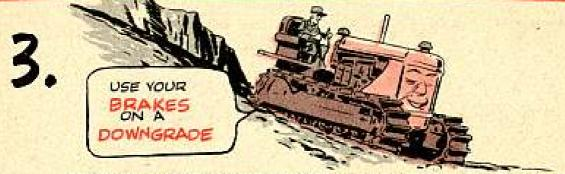
And be sure you're using the right gear, too. That load you're carrying could push the engine over its maximum speed.
