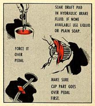
Better make sure you're not getting those pads on upside down. The flat side's supposed to fit tight against the back of the floorboard, so make sure the cup part goes over the pedal first.
