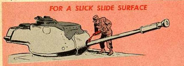
When lubricating M41, and M47 tank guns—and them only—spray some OHC (MIL-0-6083A) through the gun shield opening onto the recoil slide surface.
