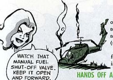
Sure, with the selector valve partially off, he'll be able to bring the chopper to a hover. But when he pours the coal to 'er, she'll flame out for lack of fuel (ugh!).
