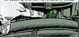
ENGINE COMBUSTION CHAMBER — Eye the housing, turbine support, exhaust collector and tailpipes for cracks, dents, burns or buckles.
