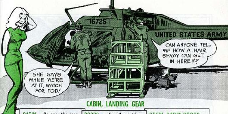
CABIN — Go over the area, looking for loose or missing rivets, cracks in the skin and other damage.
