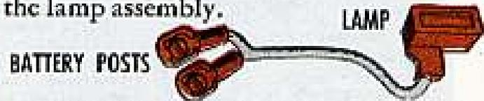
Run the 2 leads from the lamp assembly around the cradle to the BAT binding posts and secure 'em.
