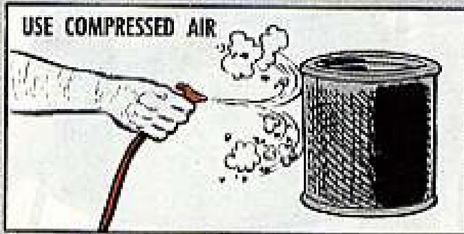
As long as you have the primary element off, give that a good airing out, too. Then clean out, and wipe out, the catch tray or bottom cup and the case that's bolted to the engine air intake. Make sure you don't leave lint or strings loose in the case.
