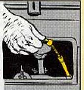
2. Clogged lubrication system. If this is the case, change the oil filter elements (FSN 2940-555-6348), clean out the filter shells, drain the contaminated engine oil, fill the engine with OE 10 and run from three to five hours. Repeat the flushing until all the sludge is washed out of the system. When it's cleared, again replace the oil filter elements and fill the engine with OE 30.
