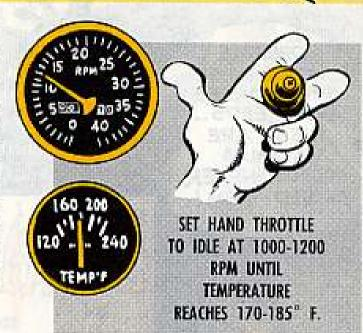
5. Stopping without cooling engine. Before engine shutdown, make sure your coolant temperature is between 170° and 185°F. If it's higher, set your hand throttle and idle between 1000 and 1200 RPM. This should bring it down to the right temperature range. If it takes longer than five minutes to cool off, then you better check out the engine like it says in Table II, item 7, TM 9-2300-216-10 or item 7, Table I, TM 9-2320-238-10.
