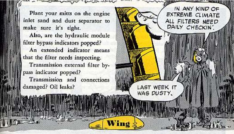
Something new has been added to an Army chopper—those "shorty" wings on the HueyCobra give additional lift and provide mounting points for the weapon's pylons. Here's what you should look for on the Daily.
