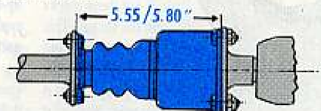
AFT SLIP JOINT SETTING
