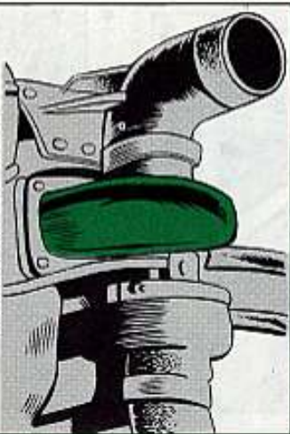
HELP YOUR TURBOCHARGER—IDLE 3 TO 5 MINUTES TO COOL.
