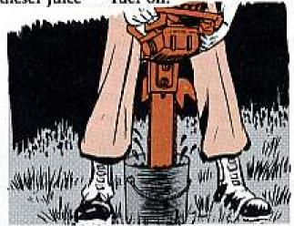
That bucket is to clean the chain when you cut rubber trees or gummy wood. Gummy sap like latex comes out with a minute or so run, with the guide bar snout dunked in 3 or 4 inches.
