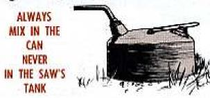
Make the mixture in the 2½-gal can you got with your saw, or in the 3-gal replacement — never in the saw's own tank. Use OE 30 non-detergent oil (OE 10 in winter), and unleaded gasoline if possible. Otherwise, use combat gasoline.
