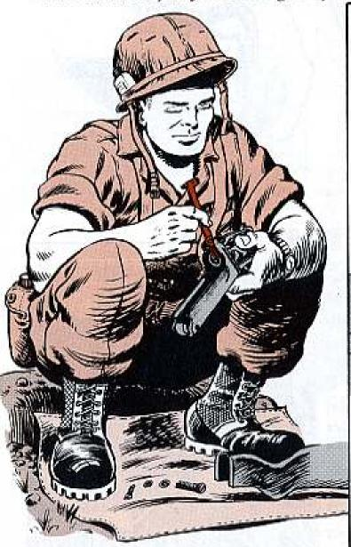
Remove the receiver group from your weapon. Then use the chisel-edge artist's brush (FSN 8020-191-3970) to work CR cleaning solvent on and around all the parts — and especially the trigger spring, hammer spring, actuator spring, latch lock spring and the like. Not forgetting the firing pin spring, either.
