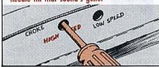
Now you're ready to make a check. Are both low-speed and high-speed needle settings close to a full turn open? If so, you've come close to a bull's eye the first shot. Open the throttle . . . do you get full power fast?
