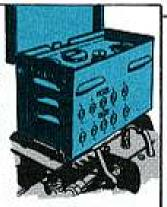
FUEL TANK—Loose on mount, leaks; strainer broken, missing; cap doesn't fit tight, tabs broken, missing, valve not open, gasket broken, missing; chain busted, missing; drain doesn't work. (Check the fuel lines, too—for leaks, sharp bends and excessive wear.)
