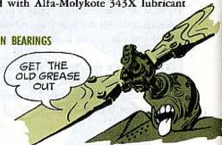
The tail rotor only twists thru a 12-degree angle during operation, which means a lot of grease in there is not being used. It can build up and harden like a rock. Then each time you purge the cavity with new grease the old grease won't budge so your grip bearings get short-changed. You know what that means—shorter bearing life . . . maybe a frozen bearing which doesn't make for a healthy situation!!
