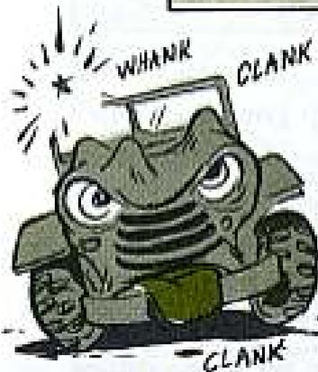
A rough-running engine may be traced to something as simple as a dirty air cleaner. Whether you've got the oil-type or dry-type, your filter has just one important duty — to keep dirt out. But air has to get thru. Your engine can't run without air. This filter needs cleaning or replacing more often in dusty operations.
