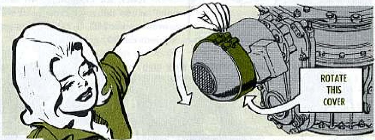
If brush cover, P/N 30010-1035, is bolted together with the opening at the top of the generator, slip the cover 180 degrees so that it's at the bottom. Then water won't leak into the generator and short out the works.
