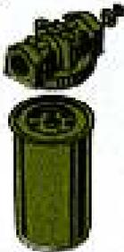
**TANK** — Leaky, mount loose, fluid contaminated, lines bent, fluid level low.
