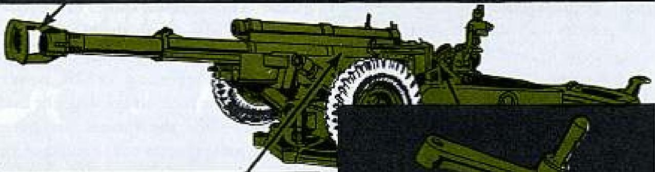
**Bore and Especially The Chamber** — A build up of material from cartridge cases really fouls 'em up. So, after every 12-15 rounds it might jam up. Use your bore brush and clean the entire bore and chamber — but good.
