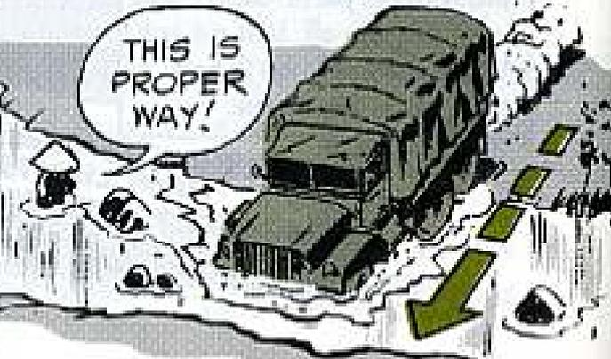
Cross a ditch or gully head-on when possible. Crossing at an angle puts a twist on the truck and even some mounted equipment. Such strain can damage the frame and just tear things apart.
