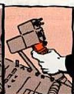
ENGINE — Check for freedom of rotation (with starter energized). Be sure the ignition system circuit breaker is "out" so the engine doesn't start when you trigger the starter. Rotate the engine for a maximum of 40 seconds. There should be no unusual noises during coastdown.
