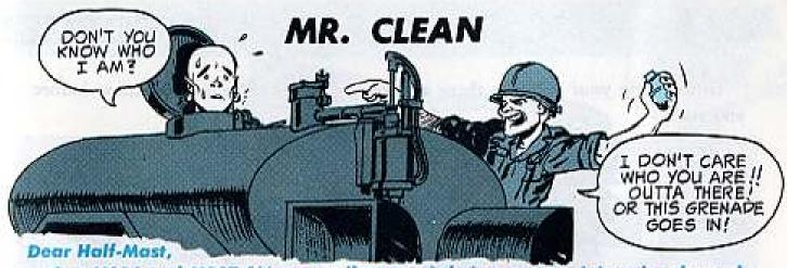
Our M106 and M107 1½-ton trailers need their water tank interior cleaned and refinished. At one time this was done by MWO 9-2330-213-30/2; now I'm told the MWO has been rescinded.
