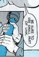
Unscrew the barrel two notches (dicks). Remove the metal link so the bolt will close.
