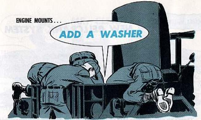
Those front engine mounts, or pads, in your 2½-ton M44A1 series multifuel ruck should last until the engine's changed. Even if the pads get mashed down so the bolt's a little loose, there's probably no reason to get shook up. You may even be able to rotate the bolts with your fingers.
