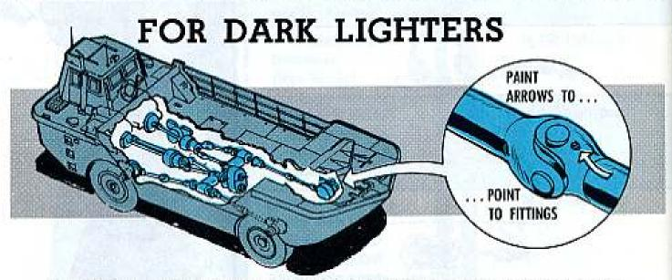
Lube joints on the LARC-V and LARC-XV drive shafts are hard to find in the dark—and the shafts have to be turned to get at 'em all.
