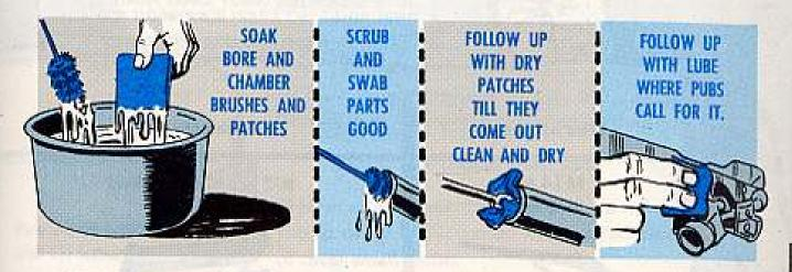
Now, no matter how careful you are shoving a wet patch through the bore, the patch is going to "squee-gee" some water into the gas system. And no matter how hard you try, you're not going to be able to drain all of the moisture out again. Result: The water that stays in there is going to cause trouble even though the gas system's metal is corrosion-resistant.
