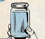
Let it set for a couple-three hours. You should be able to spot any dirt, metal or other stuff easy enough. If there's water in it, the water'll settle to the bottom.
