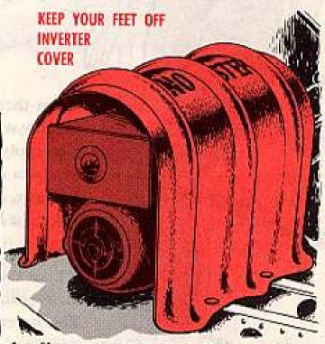
the Shawnee (CH-21) helicopter. Puttin' your manly weight on the main or standby inverters' lightweight cover could crack it up or damage the motorgenerator set.
