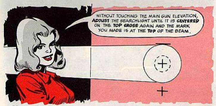
Now you have it adjusted so the light beam and the main gun hit the same target at 1200 meters.
