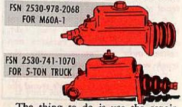
The thing to do is use the repair parts in your equipment's parts manuals. Too often, if you try a criss-cross you can wind up with a double-cross. So, stick to the book and let the Detroit engineers figure out what parts are interchangeable.
