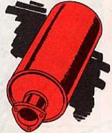
Remember, the rule whether you need a spark arrester muffler is when your truck's engine must be running while ammo's being loaded or unloaded . . . like TM 9-1300-206 (Nov 64), paragraph 71b(19) says.
