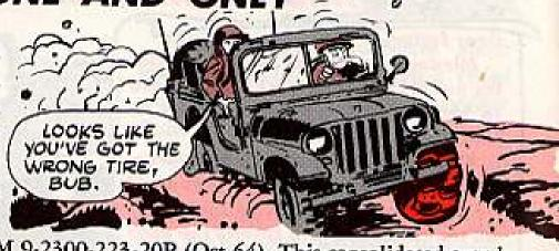
The latest word is in TM 9-2300-223-20P (Oct 64). This consolidated supply manual lists Tire, Pneumatic, 700-16, 6-ply, FSN 2610-678-1363 for all 1/4-ton trucks and trailers.
