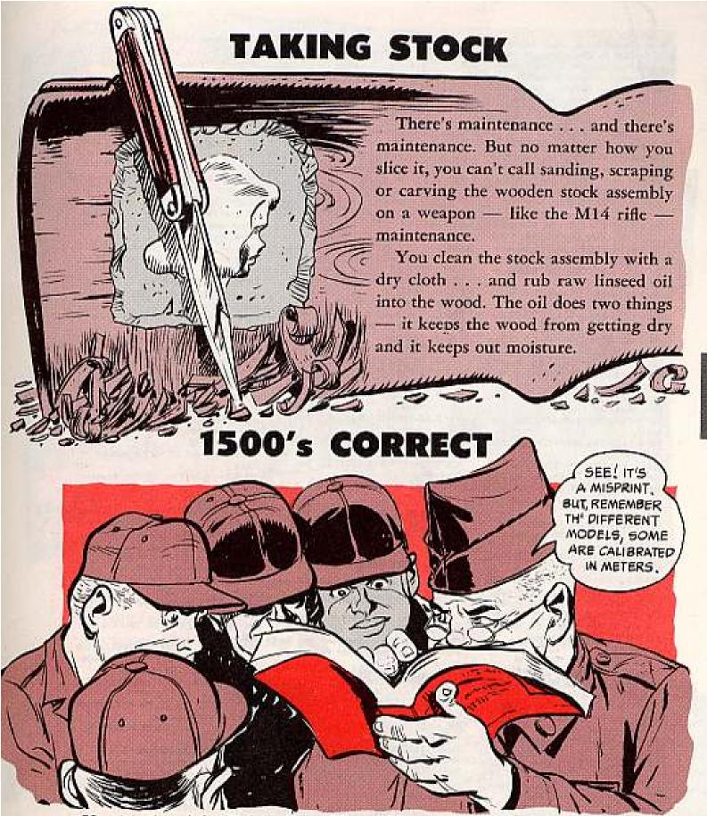
Yep, you're right, Bright Eyes. That 155 was a misprint in Item 34 of TM 9-2350-208-ESC/2 (3 Jun 64). The magic numbers for calibrating rangefinders on all M48-series tanks except the M48A3 are ± 30 and 1500. Only difference is, the rangefinders on the M48, M48A1 and M48A2 are calibrated in yards while the one on the M48A2C is calibrated in meters. On the M48A3, however, the rangefinder's also calibrated in meters, but the magic numbers are ± 30 and 1200.
