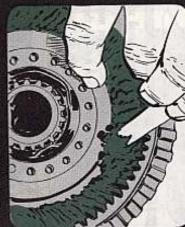
a solid coat of grease on the splines of the all the air pockets. female coupling, using a spatula to work out Now, here's where OJT pays dividends. Put
