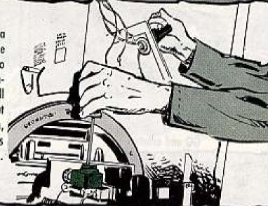
Put the FIRE gage (.020-in leaf) between the barrel extension and the trunnion block. Try to fire the gun. It should fire. As a double check, fire it again.
