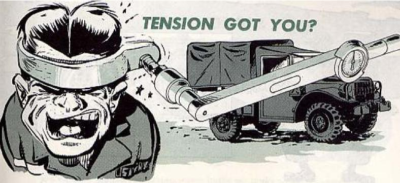
You'll have a big headache trying to use the torque wrench method of adjusting your M37-series 3/4-ton truck's fan belts if you wait till the 100-amp generator installation is all done. The belt adjustment spelled out in Ch 3 (Oct 62) to MWO ORD G741-W12 has to be done before the fan shroud and radiator are put back.
