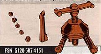
PUMP, BUCKET, LUBRICAT-ING: hand operated, 25 to 50 lb cap., 7000 psi pressure, 1/5 oz per stroke, w/10 ft Ig hose, hyd coupler, w/leakproof cover & follower pl.
