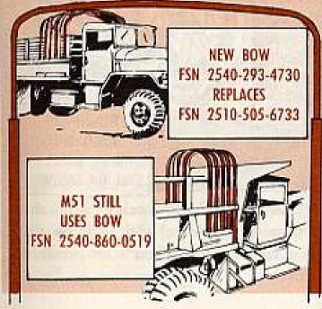
There's a new vehicular top bow for 5-ton G744-series cargo trucks. FSN 2540-293-4730 fits all models, replacing FSN 2510-505-6733 listed in TM 9-2320-211-20P (Mar 63).
