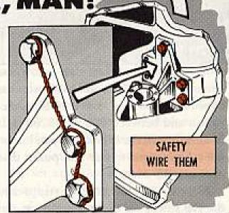
Then have 'em drill a hole in this nut (AN335-10) and safety wire it to the gear.
