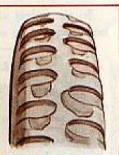
A tire that looks like this, although it shows shallow irregular wear and very little smooth worn surface, is not ready for recapping. Still got plenty of wear.
