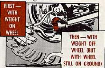
That little bit of allowable play — just when the vehicle's weight is off the wheel — is in the lower ball joint. This's because the wheel weight is on the upper joint and, besides, the upper joint is spring loaded. There's no pressure on the lower ball joint, so it will give a little.
