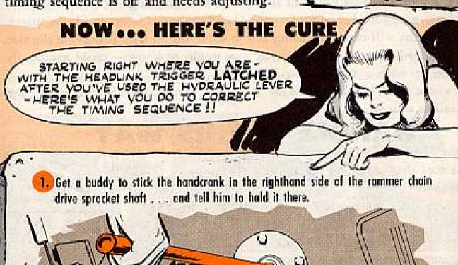
You retract the hydraulic lever and keep it retracted till the piston rod down below there stops moving. You can watch it move by looking in the rammer case. When this happens, ... your rammer chain timing sequence will be perfect. Remove and stow handcrank.
