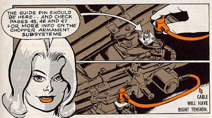
It's easy enough to put the guide pin in the right place. All you have to do is remove the four screws that hold the receptacle in the bracket . . . turn the receptacle until the guide pin is where you want it . . . and then put back the four screws.
