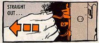
A lot of M14's are still complaining about battered ribs . . . so it looks like some guys need reminding not to rotate the trigger guard more than 90 degrees when removing the firing mechanism.
