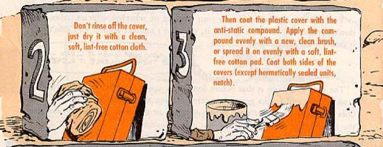
When the coating is completely dry, check the meter's anti-static protection again by rubbing the cover briskly with a soft, clean cloth. If the drying time for the compound isn't quoted on the container, let the coating dry for 30 minutes.
