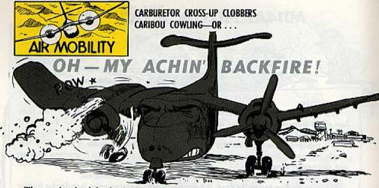
The engine backfired—just once! But that was all it took to tear up a Caribou (CV-2) cowling with the carburetor air switch in the wrong position during a start.
