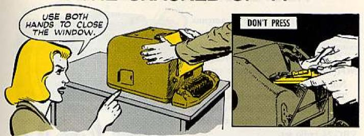
Tryin' to read copy through a cracked view window on a TT-98/FG or similar kind of teletypewriter makes for bleary eyeballs.
