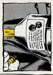
If you find anything besides fuel coming out of the secondary filter, sing out for your organizational mechanic to change both filters. It's important, especially when changing the secondary filter, to prevent dirt particles from getting into the fuel-to-injector pump.
