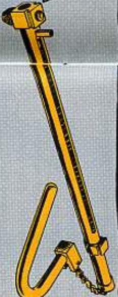
**CHARGER ASSEMBLY**—Dirty, rusty, burred, cracked, dented, twisted; detent burred, damaged; locking lug worn; charger spring rusty, pitted, worn, broken; charger handle broken, cracked; chain links worn, damaged.
