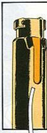
**FLASH SUPPRESSOR**—Loose; prongs and base cracked.
