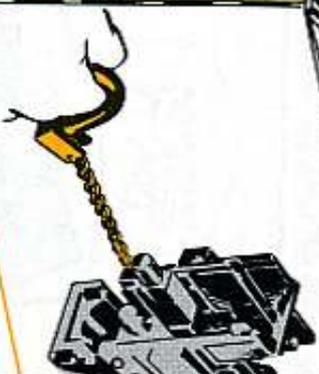
6. Now you can take the bolt out. Natch, move the feed cam out of the way, and you'll do all this in reverse to put the new bolt in.
