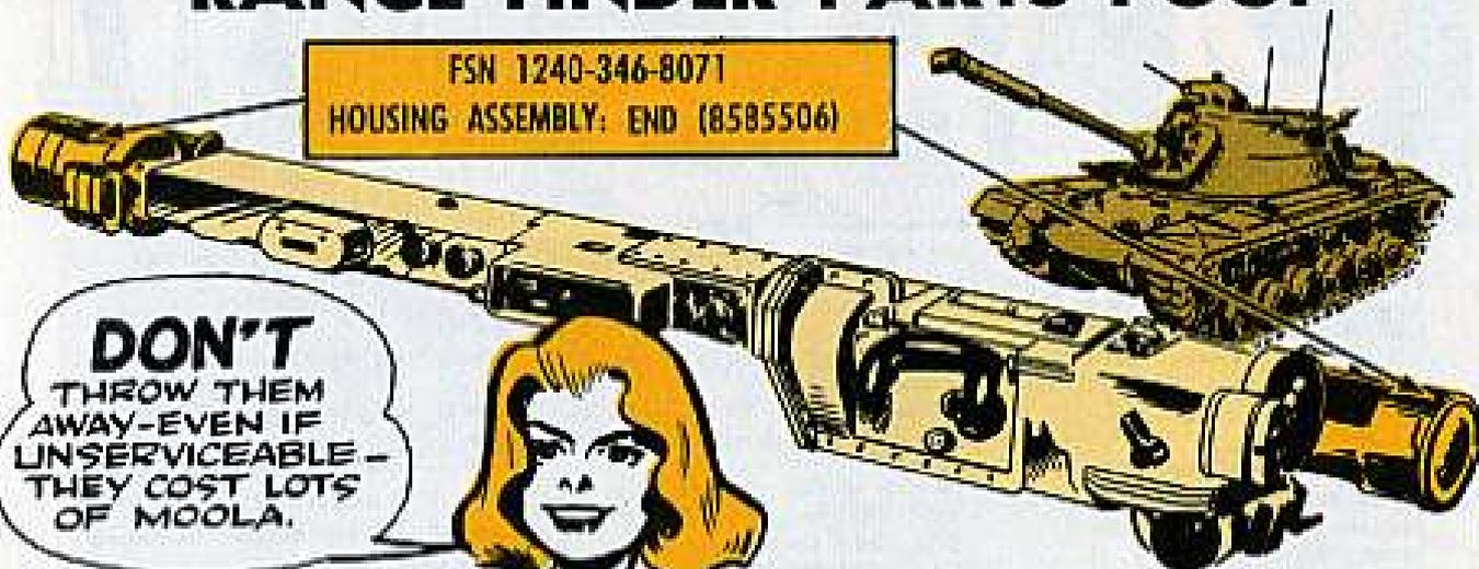
Some organizational turret mechanics have been throwing away unserviceable end housing assemblies when they replace an M17B1C rangefinder on an M48A1 or M48A3 tank.
