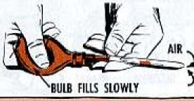
2. Put the partially filled end of the glass tube into the sampling bulb. Notice that the ½ inch yellow color in the center of the tube is the sealed color before you broke the tube ends. Yellow means there's no CO in there.
