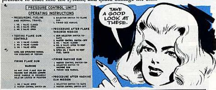
The air tanks provide a maximum air pressure of 3,000 PSI. The weapon's normal operating pressure is 325 PSI, but it'll do OK with air pressure at 250 PSI. The operating pressure can be corrected to the proper setting by adjusting the regulator valve with the key chained to the control unit.
