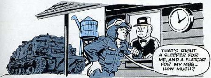
Worried about how to transport your M88 tank recovery vehicles for long distances? Well, the only way is by rail. The M15A2 draggin' wagon trailer is too short and too light. It can't haul over 50 tons maximum, and the M88 weighs 56 tons. For shorter distances road marching the M88 is the answer which means you have to keep it in top shape.
