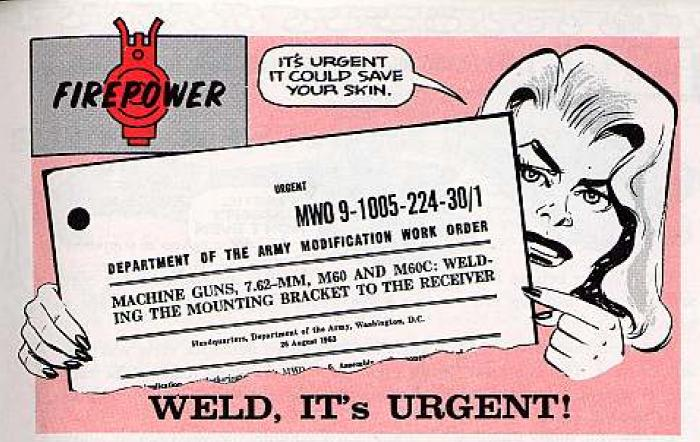
If your M60 or M60C machine gun sports any serial number from 35,500 to 37,500, make sure support gives it a treatment of MWO 9-1005-224-30/1 (26 Aug 63). This is an URGENT that welds the mounting bracket to the receiver. It'll cut down on breakage of the trigger housing mounting lug—
