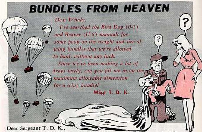
Can do. As far as weight goes, the operator's manual for the Bird Dog says you can carry 250 pounds under each wing, for a total of 500 pounds per bird. And the operator's manual on the Beaver allows you 500 pounds per wing, for a total of 1000 pounds per bird.
