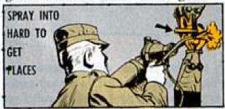
But use only enough to cover the area you're working on. Don't let the cleaner dry on the surface before rinsing, either. Otherwise it'll lose its punch.
