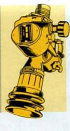
cracked, won't turn evenly, too much won't lock firm backlash; elevation worm screw burred twisted; bracket rotating knob broken burred; instrument light clamp bent, clamp cracked; wing nut busted; eye M23 TELESCOPE MOUNT — Telescope bolt bent, crossthreaded; cotter austed, rusty; clamping bolt loose,
