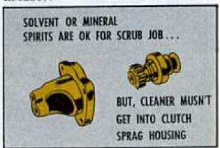
After support cleans off the gooey coat and carefully re-lubes the starter clutch area (only), you can re-claim your M60 starter and install it like your TM says.
