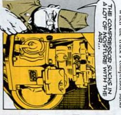
where you drivers come into the air tanks, along with the air comes a heck of a lot of moisture—and this is in the outside air and shoves it into the
