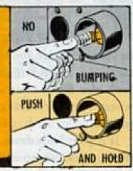
So the word on starting the 1790-2 engine in the M60 tank is: Push hard and hold. Don't bump. Half-Mast
