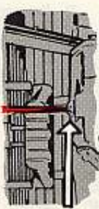
DRAINING AT OPERATING TEMPERATURE BRINGS OUT MORE SLUDGE
