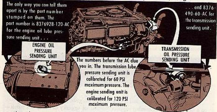
Any time an engine or transmission lube pressure sending unit gets replaced, be sure you've got the right one in the right place.
