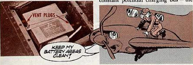
All she generally needs is the once over with a stiff fiber brush (not wire) on the case and cell tops. Should you happen to get an overcharge, gassing and bubbling of the electrolyte through the vents may give you a white film of potassium carbonate. Just brush it off.
