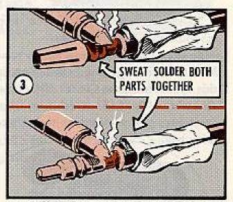
rosin core solder then sweat the two parts together. Make sure all of the naked cable ends are soldered to the terminals... not just a small portion. You need a firm and solid connection. After it cools put everything back in place.
