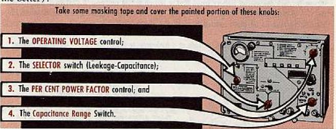
These four knobs have luminous paint which is a little more radioactive than it should be. It also tends to flake off easily—so it can stick to your hands, get carried around, swallowed, etc.
