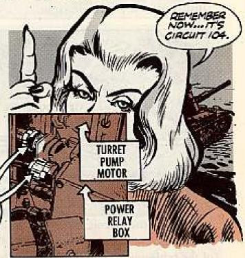
It's easy to find this circuit because "104" is stamped on a metal band around the cable. There is also a diagram of it in Fig 104 facing page 140 of your TM 9-2350-215-20 (Sep 60).
