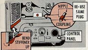
The drain plug is located about three inches back from the side of the control panel, flush with the floor of the compartment.
