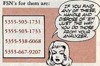
This applies only to the ZM-3A/U. The ZM-3/U does not have radioactive knobs.
