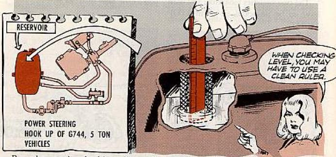
But when you're checking oil already up to this level, you may need to poke the clean end of a ruler inside the filler screen to measure it.
