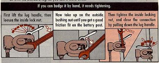
And finally, top it off with a coat of protective grease like you would with the standard lug.
