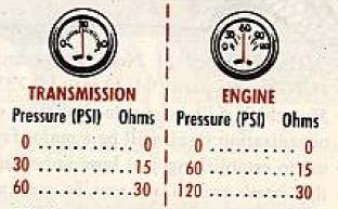
To be sure your transmission oil pressure sending unit is on the ball make these tests: Get the transmission oil warm but not hot (125° to 180°F is about right). Put the vehicle in motion. Now run it at high speed. Under these conditions lube pressures should be 40-60 PSI.
