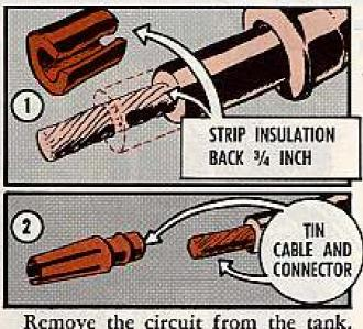
Remove the circuit from the tank. Then unscrew the nuts from both ends of the cable and sweat off the terminals. (A wet rag or some asbestos will keep the rubber from burning.) It'll be a lot easier and you'll do a better job if you strip the insulation back 3/4 inch before you start.
