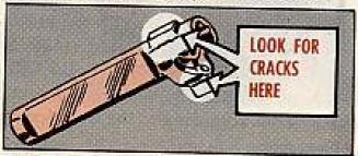
If you think a crack is making its way between the lugs and the body of the bolt, head for your armorer pronto. He'll send the carbine, bolt and all, back to your support unit if he spots a crack, or just thinks one is starting to show up.
