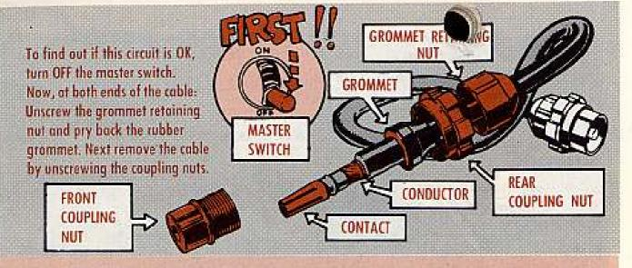
Now look over the solder joint. The insulation should be stripped back for enough to leave about \( \s\) inch of the conductor exposed. If you can see a smooth, shining, fillet of solder between the end of the contact and the exposed conductor and you can't pull the contact and the conductor apart with an easy pull, your cable is probably OK. Otherwise, better play safe and resolder it.
