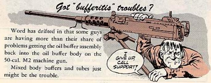
Could be that the last time the weapon was checked out by support somebody pulled a rock and joined a new type tube with an old style buffer.
