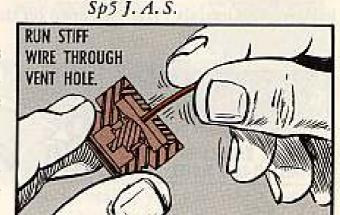
If the battery's bulging with its vent holes open, here are some possible causes: Battery box drain holes and vents may be sealed so the battery can't breathe.
