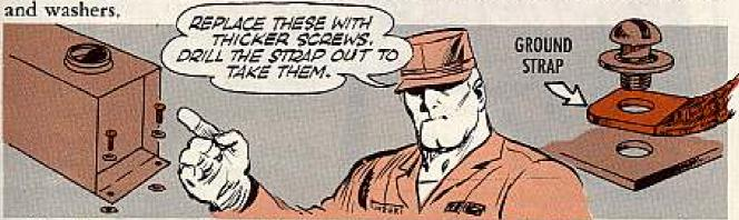
You'll have to make the hole in the ground strap a mite bigger—from \( \frac{1}{16} \)-in to \( \frac{1}{4} \)-in—to take the \( \frac{1}{4} \)-20 screws.
