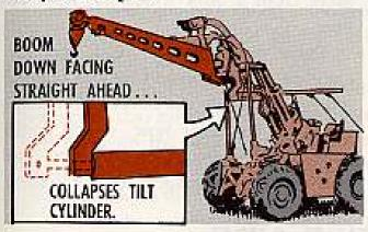
Park your MR-100 with his boom down and facing straight ahead. This'll collapse the tilt cylinder and help protect it against the weather.
