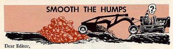
When we're working on a range job, I've noticed that sometimes in the fill or dumping areas, the ground'll get rough or wavy with a hump and then a trough. This is usually the result of dumping while traveling too fast. Once this starts, each load that follows carries the roughness and the humps further along.
