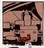
And park your NC-10 with the boom down and facing all the way to the right, if you possibly can. This'll close the swing cylinder piston rod so's the weather can't get at it.
