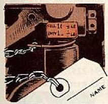
Using your scale, weight your portable extinguisher "as is." Subtract the weight of the cylinder EMPTY remember, you will find that figure stamped on the cylinder.
