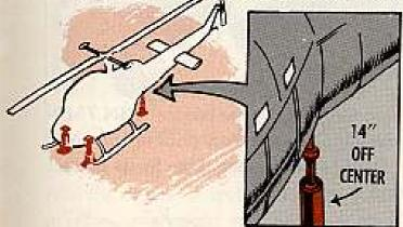
within the allowable CG limits—but it molest choppers than vice versa, your sure does not add to the bird's stability best safety approach is to rope off the on jacks.
