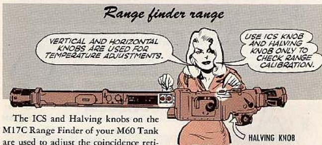
The ICS and Halving knobs on the M17C Range Finder of your M60 Tank are used to adjust the coincidence reticle like it says on pages 71 to 73 of TM 9-2350-215-10 (Jun 60). After you get the reticle adjusted, the red shields are locked into place over the two knobs to remind everybody KYCPHOI—Keep Your Cotton Pickin' Hands Off It—until your reticle has to be adjusted again.
