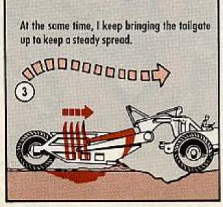
Travel fairly slow while you're cutting and spreading. You may have to go over the same spot two or three times since the dirt may compact and there can be small hollows where the dirt was spread.
