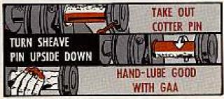
And don't forget to replace the pin.
