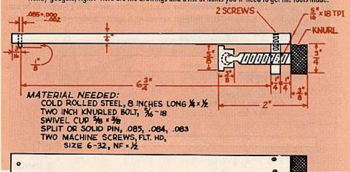
If you run into a roadblock on getting this extractor tool made, you can improvise and come up with an extractor rig that's easier to make and one that'll get the job done just as well. F'rinstance, just to get you started on the right road, here's what can be done with a hunk of steel, a common  $\lambda_{16}$  nut and bolt, a wing nut and a little brazing and welding. The spring-plunger tool is the same—no matter which extractor tool you have made.
