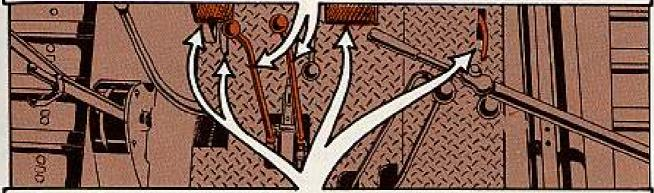
When you have icing conditions—you lock or block the rig for parking any way EXCEPT by locking the steering brakes. You can really tear up the peapatch trying to move out with brake bands frozen to the drums.
