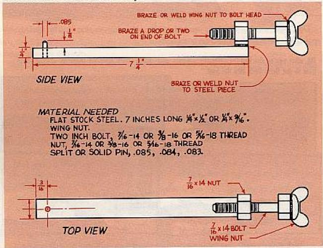
If you use this idea—and it works just like the other one—don't forget to braze a coupla drops on the tip of the bolt—it serves as a softer buffer—and keeps you from banging up the M60 bolt plug.
