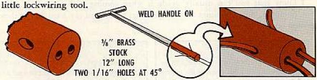
The tool is made of 1/8-in brass stock, 12 inches long. On one end you weld a handle. On the other end you drill two 1/16-in holes at a 45-degree angle.
