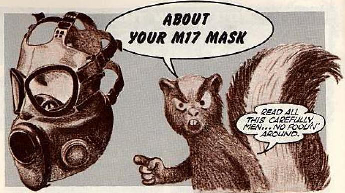
Your M17 protective field mask does not have a canister but it does have filter elements instead.
