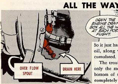
When you drain it, drain it all the way. That's the word on the Beaver (L-20) engine drain box.
