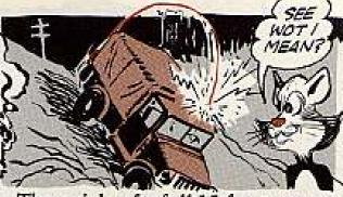
The weight of a full 15-foot antenna is enough to make it droop all the way down to the wet tarp on the vehicle—if the angle of the truck is enough.
