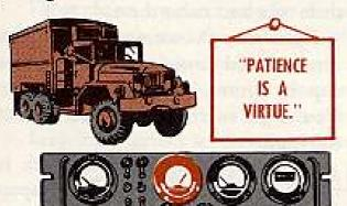
Some kind of reminder sure is needed to make sure you don't shut down the 115-volt motor generator before the 400-cycle voltmeter on the indicator panel reads less than 30 volts. When you shut down the generator before the voltage drops below the 30 figure, the control voltage is taken out of the controller before the 400-cycle power has fallen off. This sets the controller to running . . . and it keeps going till the 400-cycle power dies down.
