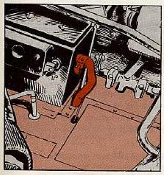
gettin' disconnected and connected every so often. So it starts to sag into the rudder cable, which rubs away at the drain hose on your bird until the chafing wears out the hose.
