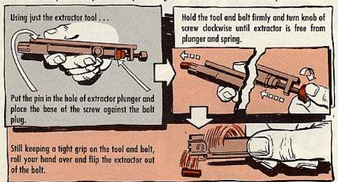
To release the spring and plunger, make sure the open end of the bolt is held tight against a table or desk. Then turn the tool knob counter-clockwise until spring snaps out. MADE EASY
