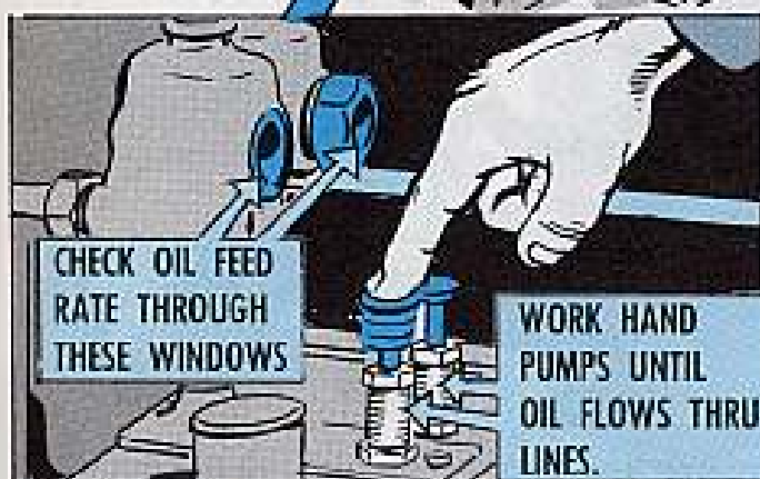
3. Stroke the hand pumps again until oil flows from the oil lines. Then reconnect the copper lines to the oil check valves.
