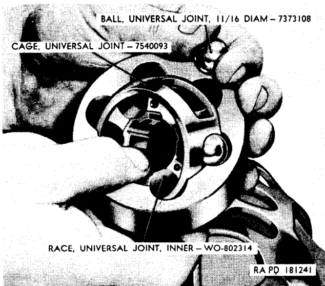
Figure 105. Installing front axle Rzeppa universal joint ball.
