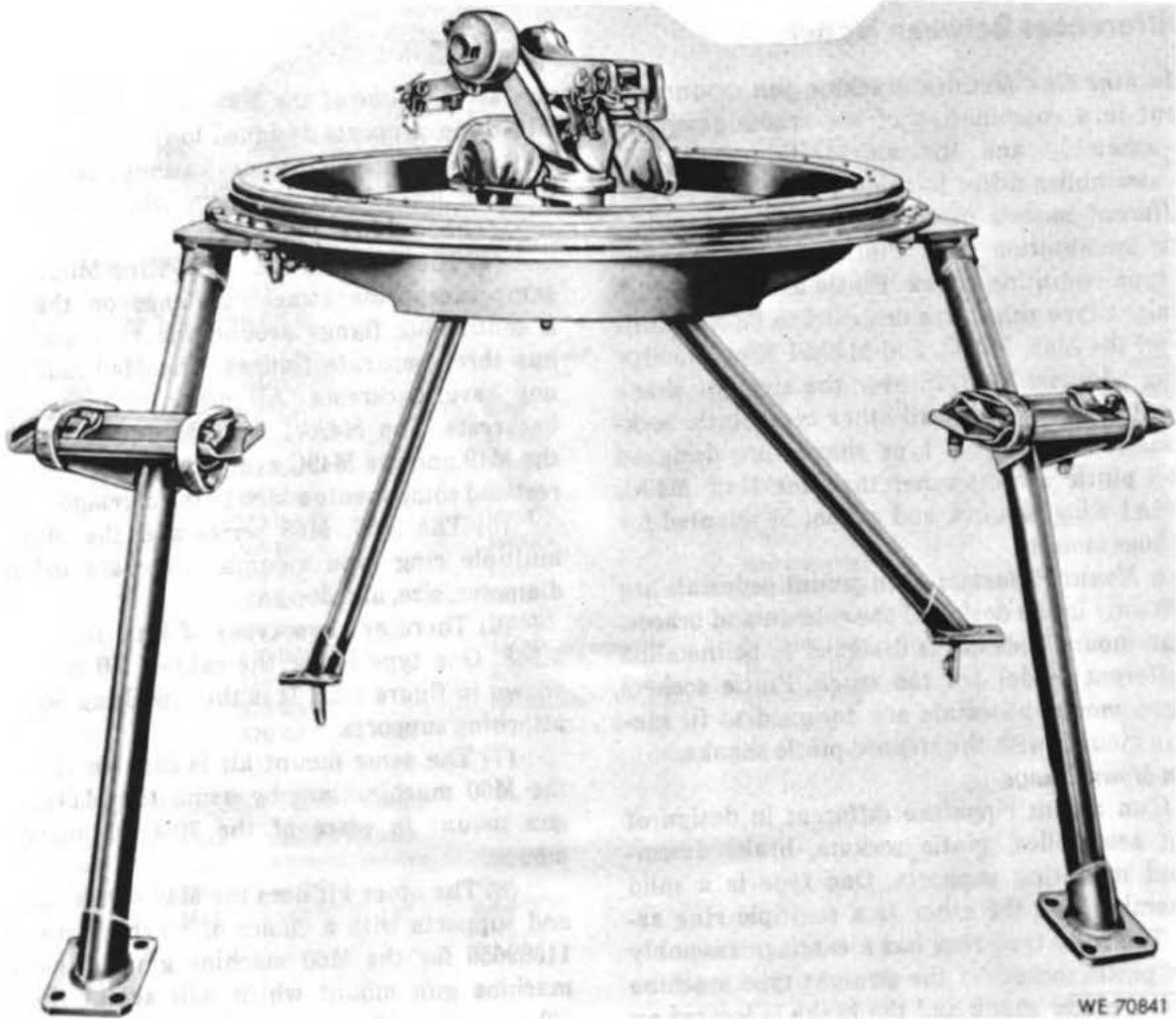
Figure 1-21. Mount, gun, ring = 11631740 (Cal. 50 M66 type ring for carrier M548).
