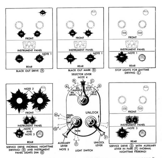
NOTE 1. STOP LIGHT GOES ON WHEN BRAKES ARE APPLIED
